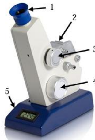
Fig. 1. The Abbe Refractometer: 1-eyepiece with scale; 2-upper illuminating prism; 3-dispersion correction knob; 4-setting knob; 5-thermometer
