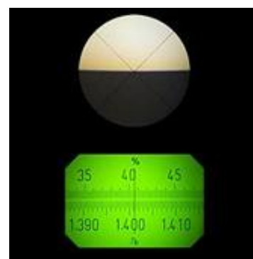
Fig. 2. The field of view in the eyepiece of the Abbe Refractometer
