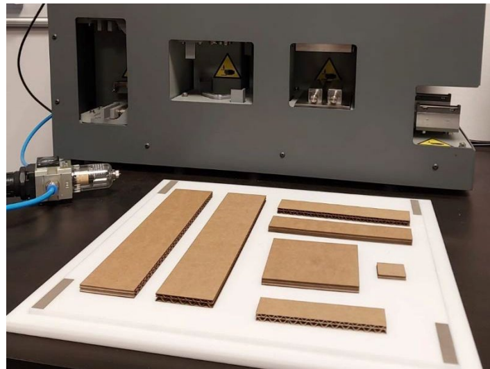
Figure 2. Material testing procedures: single set of cardboard samples and strength testing machine in the background.
