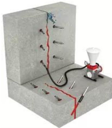
Fig. 9. Pressure injection of cracks
