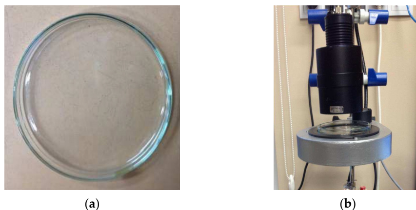
Figure 1. A sample of the training set; (a) a mixture of propionic acid and distilled water in a Petri dish; (b) a spectrophotometer with an RP-7 probe.
