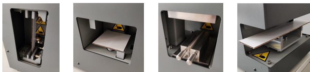
Figure 5. Testing sockets of the measuring device used for determining the mechanical properties of corrugated cardboards (from left: torsion, transverse shearing, ECT, and four-point bending) (source: authors' own work).
