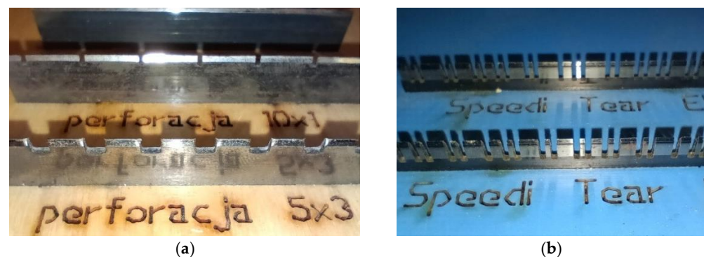
Figure 1. Knives for (a) 10 \times 1 mm (upper) and 5 \times 3 mm (lower) standard perforations and for (b) Speedi Tear perforations.
