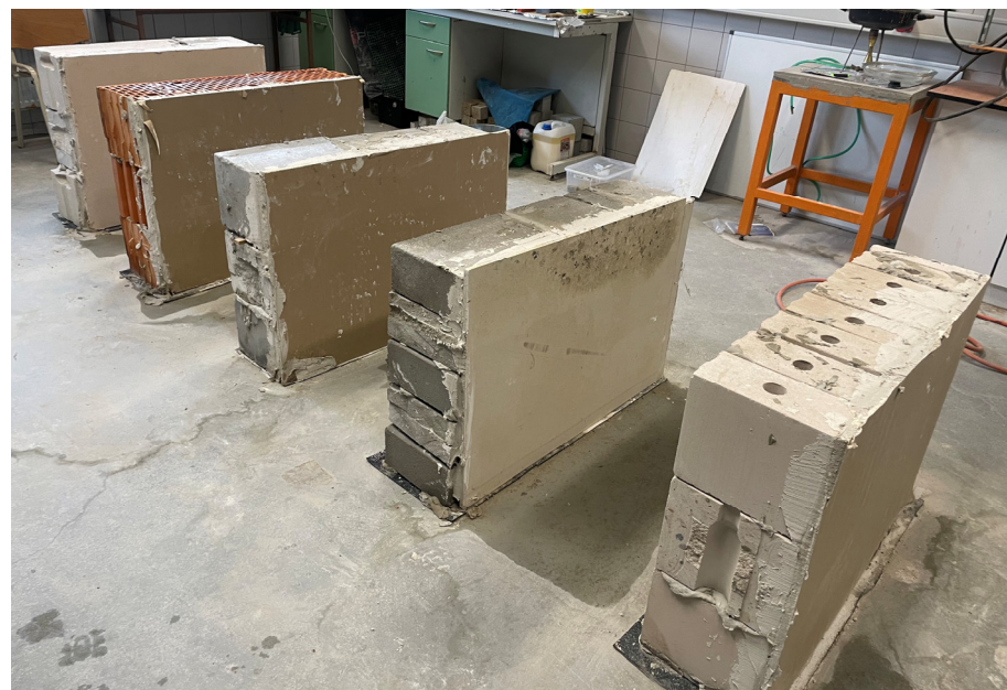
Figure 1. Walls selected for the study. From left to right: wall made of autoclaved aerated concrete, wall made of ceramic hollow blocks, wall made of perlite concrete, wall made of concrete blocks, and wall made of Sika sand–lime blocks.
